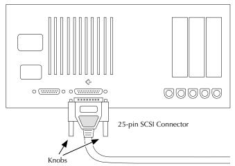
3. Attach the other end of the cable to either of the identical SCSI ports on the back of the Scanner. Seat the connector firmly and pinch the thin wire clamps shut.
